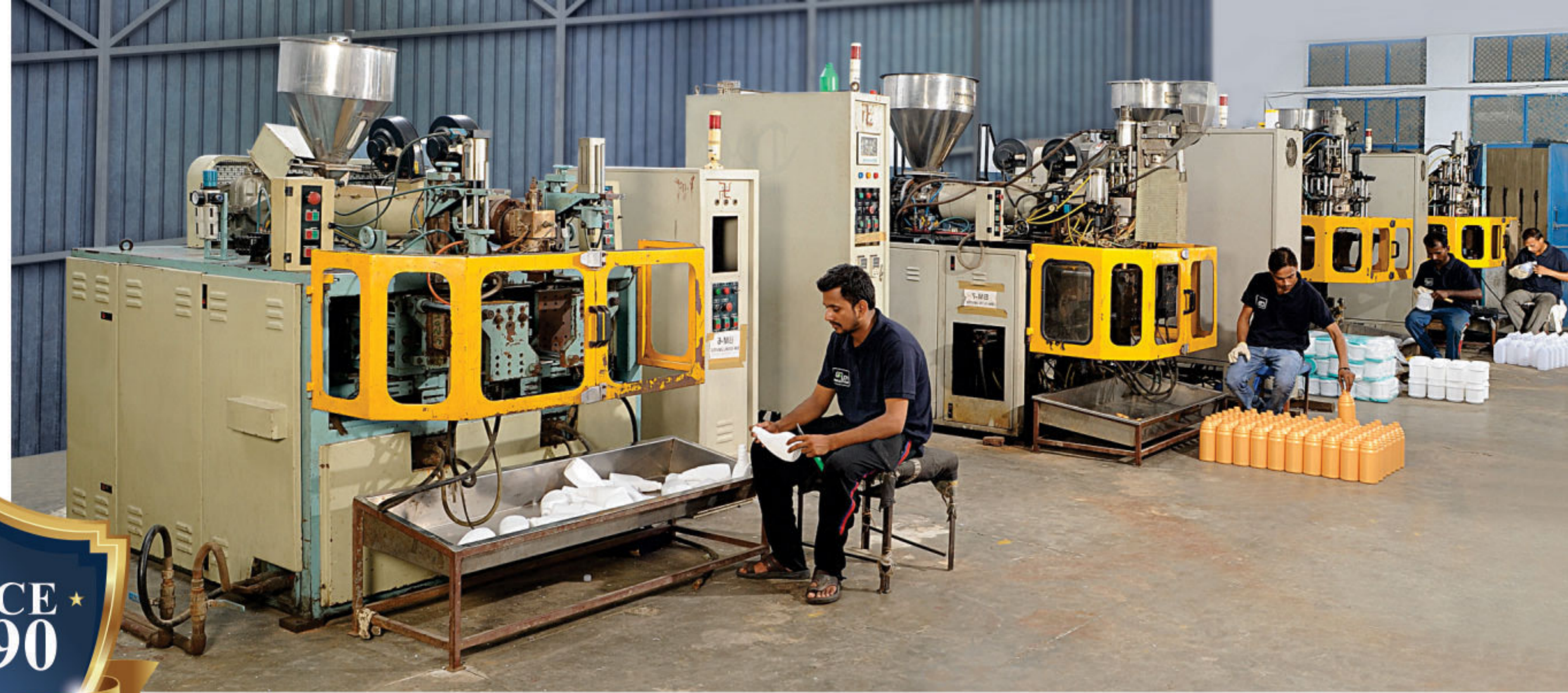
BLOW MOLDING MACHINE FOR PACKAGING - 50ml to 3 Ltrs.
