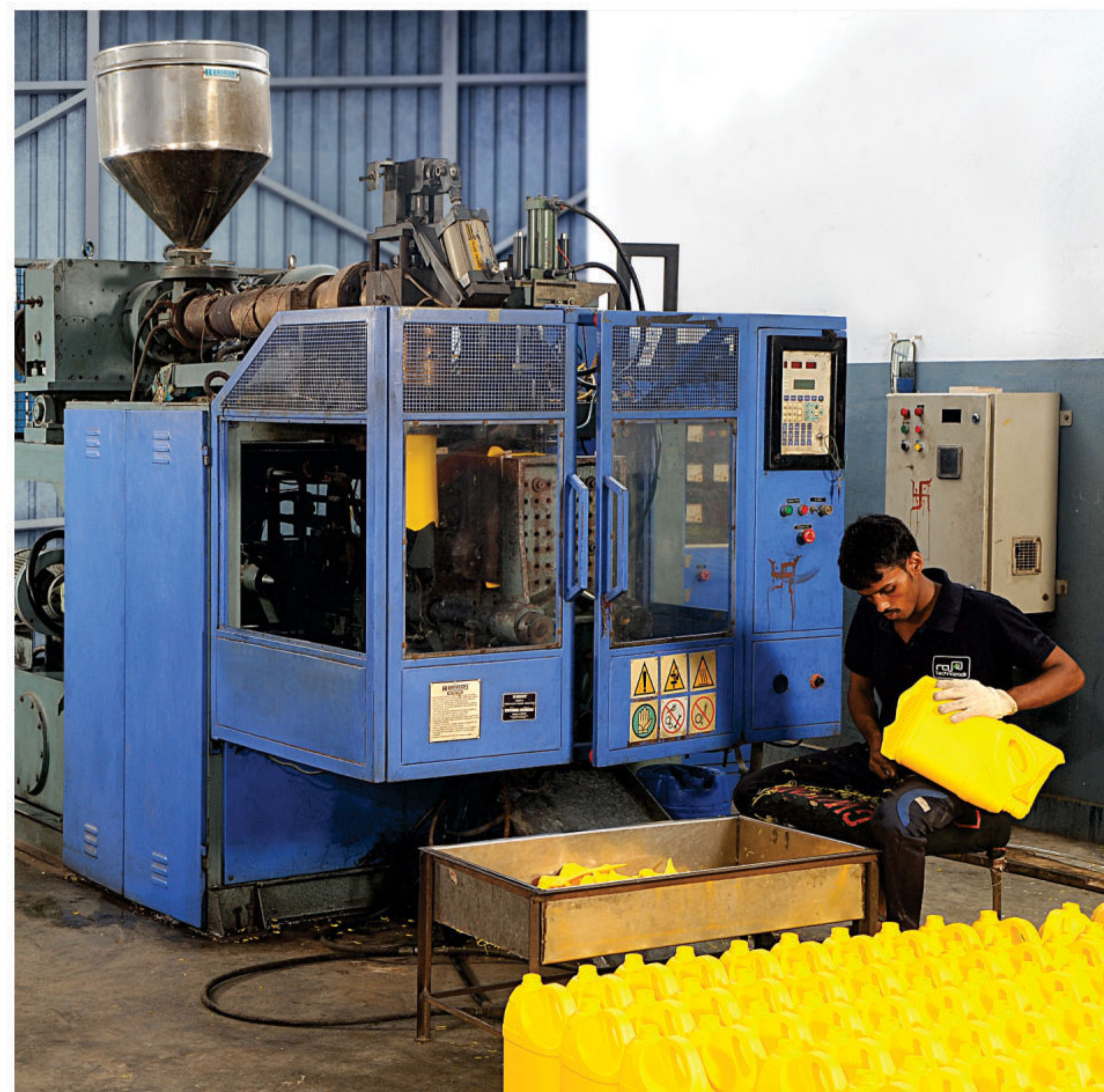
BLOW MOLDING MACHINE FOR THE PACKAGING OF 5 Ltrs. to 120 Ltrs
